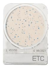
CompactDry ETC is based on the usage of X-glucoside (X-Gluc) and selective antibiotics. Enterococci beta-glucosidase targets X-Gluc and allows the specific detection of enterococci through the formation of blue to blue/green colonies.
