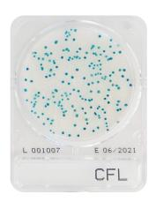
CompactDry CF-L is a ready to use dehydrated media plate used to detect coliform bacteria in dairy products such as cheese, milk, yogurt, and any products containing lactic acid bacteria. It is specifically formulated to counter the negative effects of lactic acid bacteria on chromogenic substrates. Coliforms colonies are blue to blue/green.
