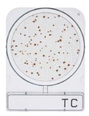
CompactDry TC is a medium containing nutrient standard agar and is used for total viable bacterial count. Bacterial colonies are coloured red due to the redox indicator tetrazolium salt.
