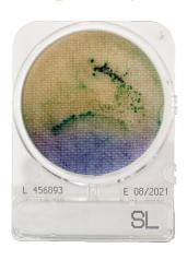
CompactDry SL detects salmonella using a 20 – 24 hour pre-enrichment step. The plates are based on the combination of different test principles:
