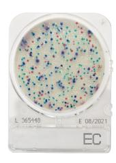
CompactDry EC is a medium to detect *E. coli* and coliform bacteria. The medium contains two different chromogenic enzyme substrates: Magenta-Gal and X-Gluc. *E.coli* forms blue colonies. Red and blue colonies counted together provides the total coliform number.
