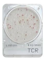
CompactDry TCR is a rapid medium containing nutrient standard agar and is used for total viable bacterial count. Bacterial colonies are coloured red after 24 hours of incubation due to the redox indicator tetrazolium salt.
