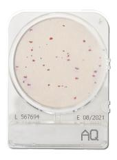
CompactDry AQ plates contains a chromogenic nutrient poor medium for determining the colony count of heterotrophic organisms in treated drinking water and ultra-pure water. Colonies are almost all red. Yeast tends to grow as white-pink colonies. Mould grows in a typical 3-dimensional "cotton wool" form.
