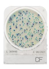
CompactDry CF is an easy tool for the detection of coliform bacteria. The media contains the chromogenic enzyme substrate X-Gal and coliform colonies are coloured blue/blue green. The growth of other bacterial types (genius) are mostly inhibited, but in certain instances may form colourless colonies.
